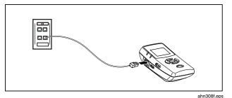
Figure 2-4. Single-Ended Connection into a Wall Jack.
