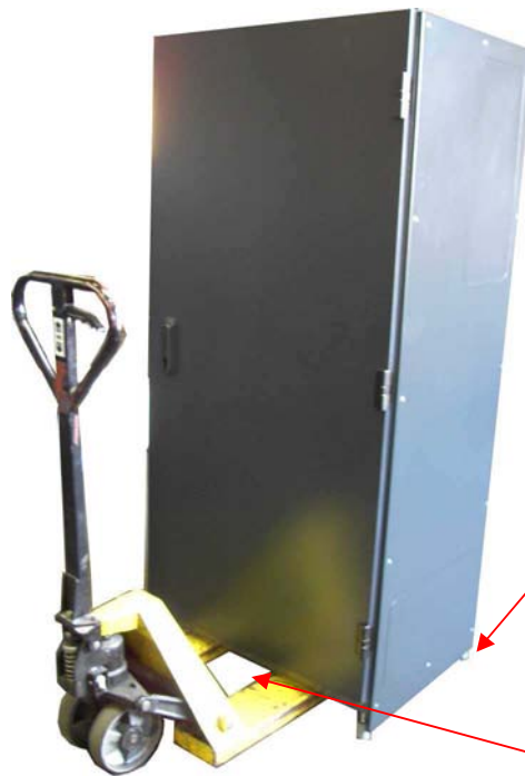
Photo: Handling by low platform lift truck
