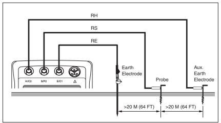
Figure 4. Three-Pole Measurement Setup
