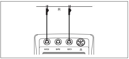
**Figure 5. AC Resistance Measurement**
