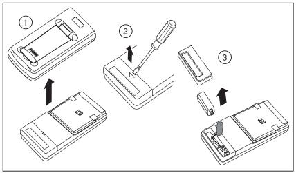
Figure 3. Battery Installation
