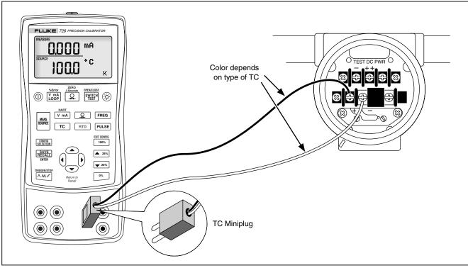
Figure 16. Connections for Simulating a Thermocouple
