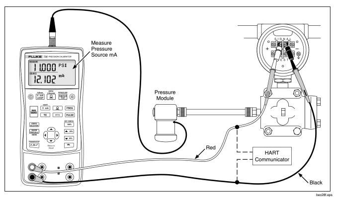
Figure 22. Calibrating a Current-to-Pressure (I/P) Transmitter
