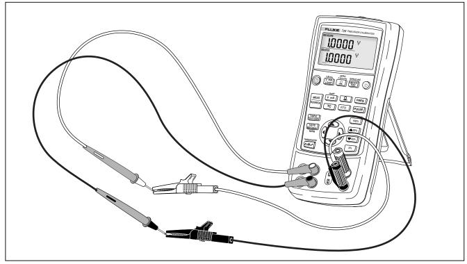
Figure 6. Voltage-to-Voltage Test
