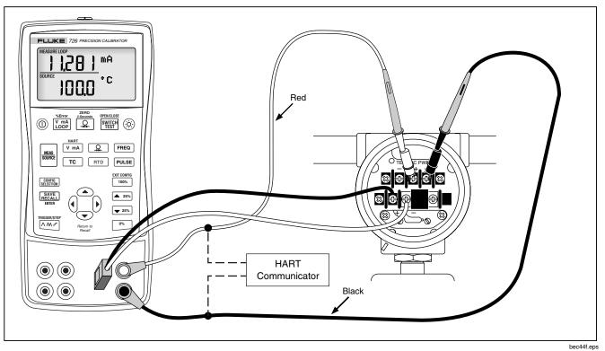
Figure 20. Calibrating a Thermocouple Transmitter
