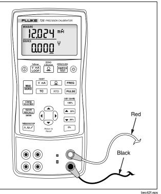
Figure 7. Measuring Voltage and Current Output
