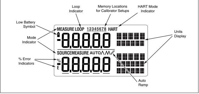
Figure 4. Elements of a Typical Display
