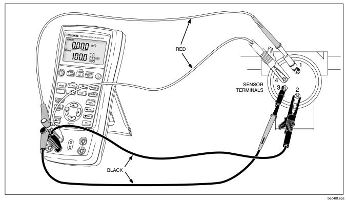
Figure 17. Connections for Simulating 3- and 4-Wire RTD
