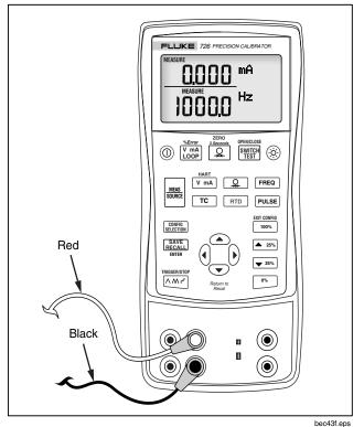
Figure 9. Measuring Electrical Parameters
