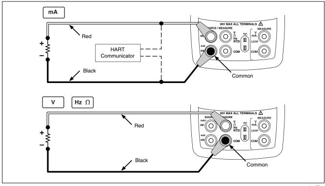
Figure 15. Electrical Sourcing Connections
