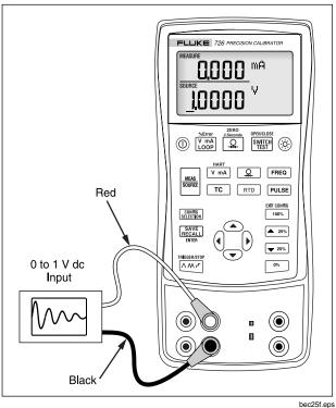
Figure 23. Calibrating a Chart Recorder
