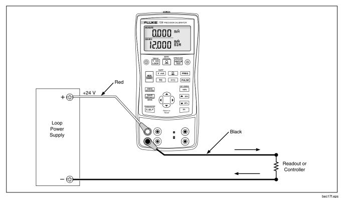
Figure 14. Connections for Simulating a 4- to 20-mA Transmitter
