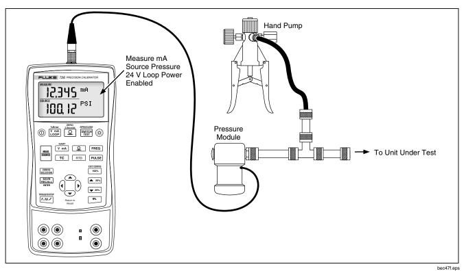
Figure 18. Connections for Sourcing Pressure
