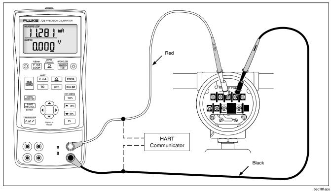
Figure 8. Connections for Supplying Loop Power
