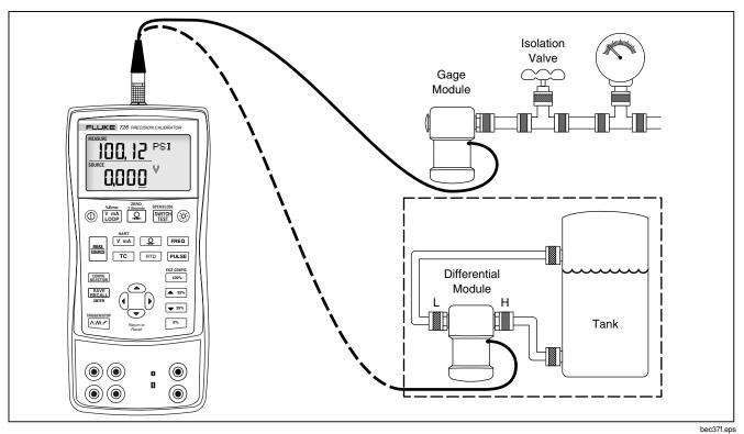
Figure 13. Connections for Measuring Pressure
