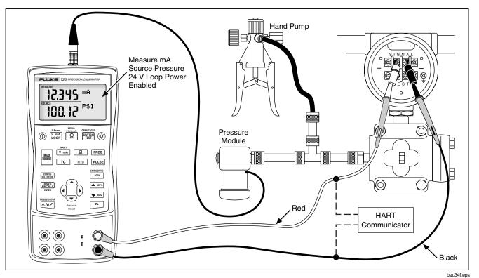
Figure 21. Calibrating a Pressure-to-Current (P/I) Transmitter
