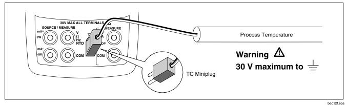
Figure 10. Measuring Temperature with a Thermocouple
