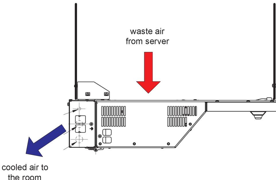
The warm server waste air is cooled by heat exchanger to about 22°C / 71°F, before it is fed into the installation room. The cooling water is provided by a chiller made available on site.
