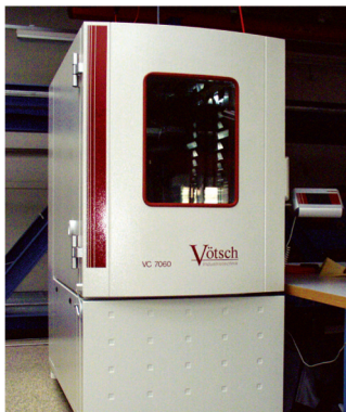
Climatic test cabinet for cyclic and ageing tests.
