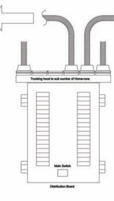
Prefabricated and modular wiring systems
