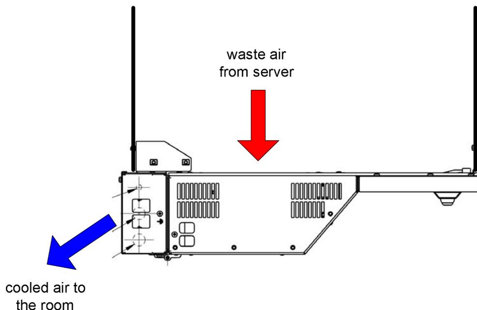
The warm server waste air is cooled by heat exchanger to about 22°C / 71°F, before it is fed into the installation room. The cooling water is provided by a chiller made available on site.
