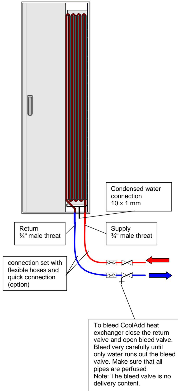
The cooling water pipes have to be insulated to avoid condensation and losses using a waterproof isolation.
