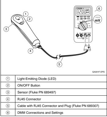
Fluke CO-210 Carbon Monoxide Probe
