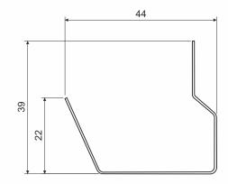
product description: it is used to divide the interior of the trunking, thus allowing a better manipulation with the inserted cables and clarity is fixed with PSK 1 to the trunking systems individual partition walls should be connected with PLSK connecting wire
