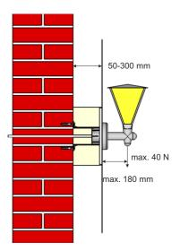
There is necessary to cut the carrier including inserted insulation before installation depending on layer thickness insulation.
