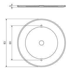
product description: to cover the boxes with fixing spacing of 60 mm using fastening screws for premises with increased need for protection of persons and property
