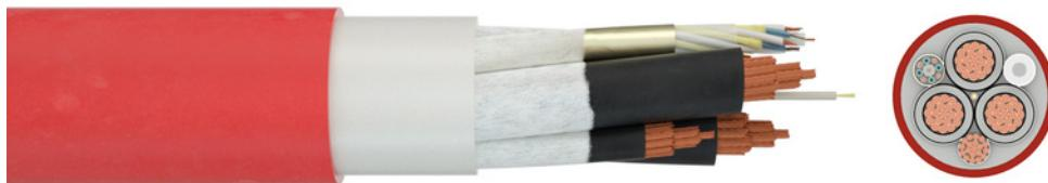
**Application:** The cables are suitable for use in high voltage shore connection systems (HVCS), on board the ship and on shore, to supply the ship with electrical power from shore, using control cores and fiber optics to adapt different type of vessels. The cables can be manufactured to order or project-specific with E9/125, 50/125 or 62.5/125 fibres.
