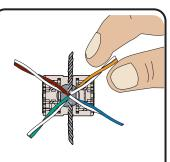
Arrange pairs in an "X" being sure to follow wire map on termination cap.
