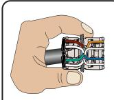
Inspect cap for correct wiring and lacing of conductors. Be sure foil or braids and all conductors are fully seated into slots as shown.
