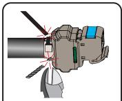
Tighten tie wrap. Trim excess tie wrap and braid pigtail.
