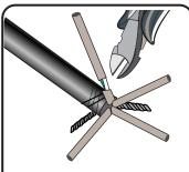
Carefully, put a starter cut into the foil as close to the center of the "X" as possible.
