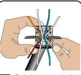
Push wires one at a time into the wire guides.
