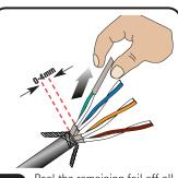
Peel the remaining foil off all four pairs. At this time all pairs should be exposed.
