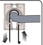
Insert tie wrap into termination cap using slots in cuff.
