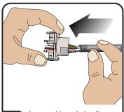
Insert cable and pigtails through the center opening of the termination cap until it bottoms out.
