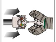
Insert the termination cap with the shield guide post aligning with the channel in the termination cap cuff.
