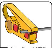
Using a Siemon ALLPREP™ tool or equivalent remove approximately 38 mm. (1.5 in.) of sheathing.
