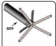
Separate shielded pairs into an "X" shape.
