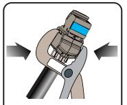
Using pliers, squeeze the shield case together.
