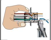
After all wires are in place trim off excess wire as close to the cap as possible.
