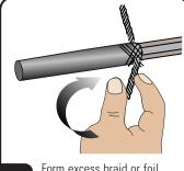
Form excess braid or foil into 2 pigtails.
