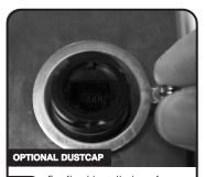
For fixed installation of optional dustcap (X-CAP) place securing ring over the outlet and flat against the faceplate
