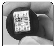
View the color code label on the outlet to determine the proper location of conductors based on preferred wiring scheme.
