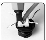
Align cable jacket into the center of the S310® block so that the cable jacket will extend within the termination cap. Lace the four pairs into the S310 block according to the color code. On a flat, clean surface, use the S814 impact tool or equivalent on low setting and punch down the pairs to terminate.
