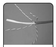
Fan out cable to desired wiring scheme. If present, cut the pair isolator as close to jacket as possible.
