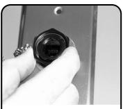
Place the panel nut over the flange and tighten to 1.69-2.26 N-m (15-20 in-lbs).
