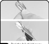
Peel the foil shield away from the twisted pairs.
