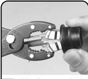
Using pliers, squeeze the shield case together until latched.
