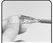
Form the pairs, foil, and drain wire into a single piece.
