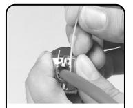
Insert the tie wrap into the termination cap through slots in the cap. Tie wrap should form a "U" shape inside the cap.
