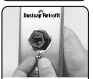
To retrofit optional dustcap (X-CAP) place the securing ring over the panel nut flush to the faceplate. Rotate the securing ring 1/8 of a turn.
