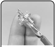
Insert pairs, foil, and drain wire through the center opening of the termination cap and push termination cap against the cut surface of the jacket.
