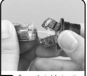
Prepare the jack for insertion by opening the shield case.
