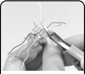
After all wires are in place, trim off excess wire as close to the cap as possible using Siemon diagonal cutters (P/N: CI-CUTTER) or equivalent. Inspect the cap for correct wiring and lacing of conductors before proceeding.
