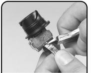
Tighten the tie wrap. Trim excess tie wrap, foil, and drain wire.
