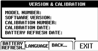
The screen gives you information about the model number with software version, the calibration number with latest calibration date, and the latest battery refresh date.
