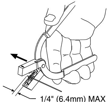
**6. Cleave 900 $\mu$ m Tight-Buffered Fiber**
