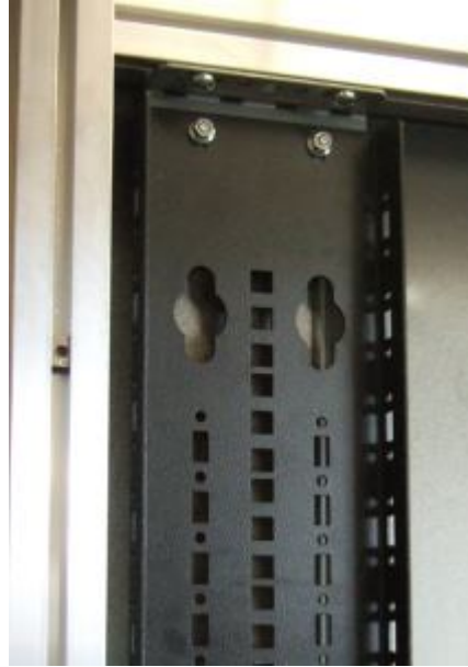
Installation to the 19" extrusion
