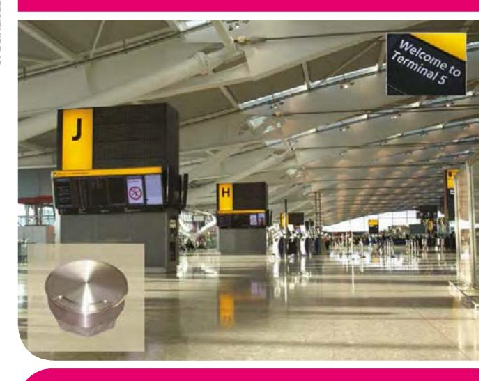
Working closely with SPIE Matthew Hall and BAA, Marshall-Tufflex collaborated to produce rectangular, round and square floor boxes in various sizes. Many of the boxes have lockable lids and all are fabricated in heavy duty stainless steel to take higher point load than standard floor boxes, enabling them to cope with wheeled traffic and protect the cables within. The boxes accommodate Cat 6 cabling with provision for Cat 7 and Cat 7a systems.
