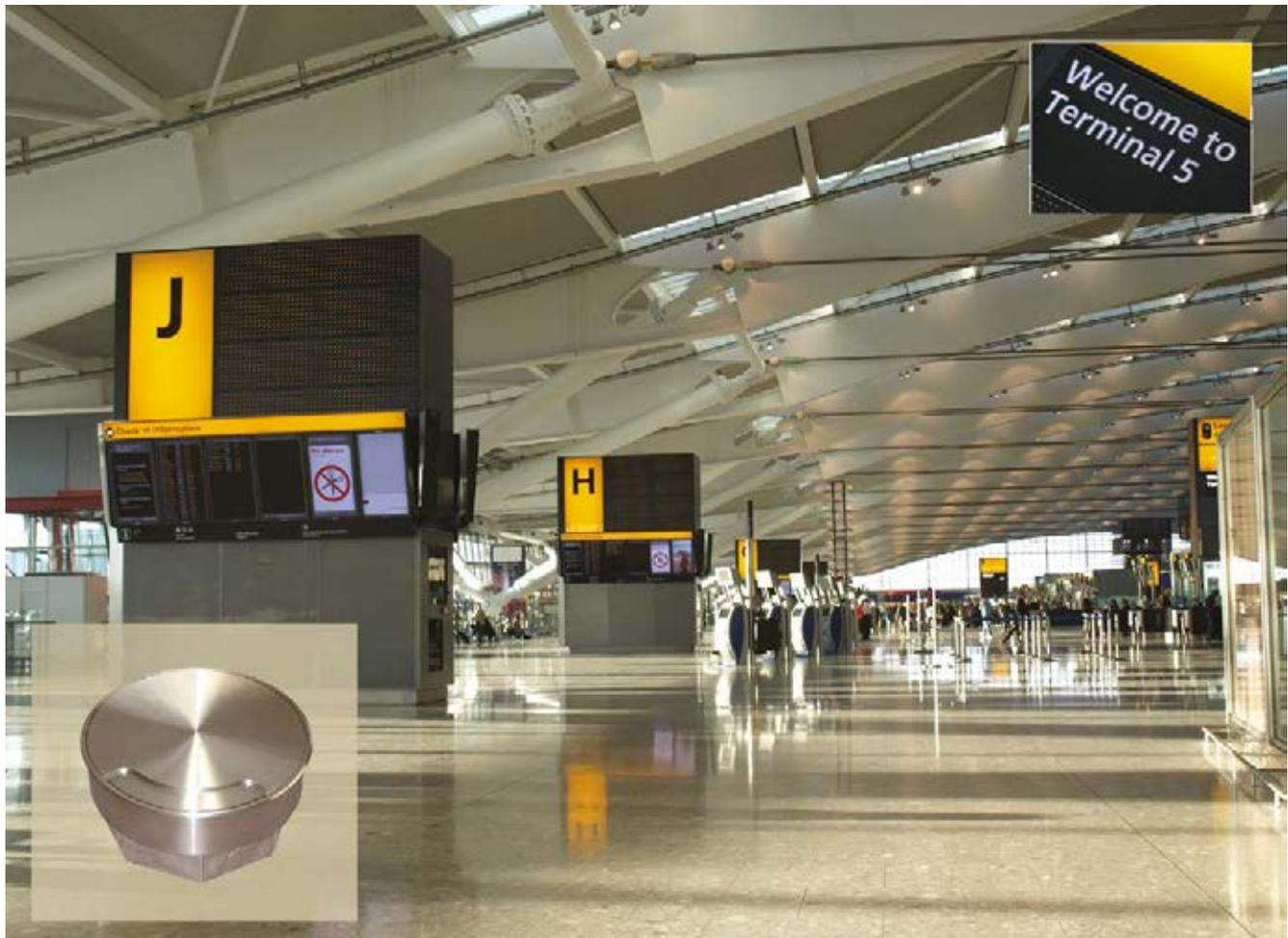
Working closely with SPIE Matthew Hall and BAA, Marshall-Tufflex collaborated to produce rectangular, round and square floor boxes in various sizes. Many of the boxes have lockable lids and all are fabricated in heavy duty stainless steel to take higher point load than standard floor boxes, enabling them to cope with wheeled traffic and protect the cables within. The boxes accommodate Cat 6 cabling with provision for Cat 7 and Cat 7a systems.
